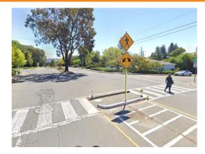
**DESCRIPTION:** Install Rapid rectangular flashing beacons (RRFB) at this intersection including minor lane configuration. The City will apply for HSIP cycle 12 grant from the State due Sept 2024. The application will include a concept plan and preliminary estimate.
