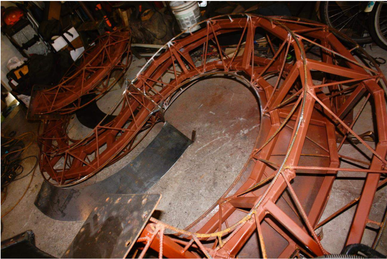
Here is a photo of the internal structure of one of my sculptures. This is before I add the corten steel sheeting. You can see one of the panels in the middle left of the photo before it is welded on.
