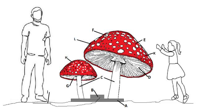
**A** - **Steel plate**. Designed with mounting holes to be bolted to concrete pad, or can be placed on a prepared compacted earth, or buried under the soil to make the sculpture more integrated into the earth. Approximate size will be 4' x 6'.
