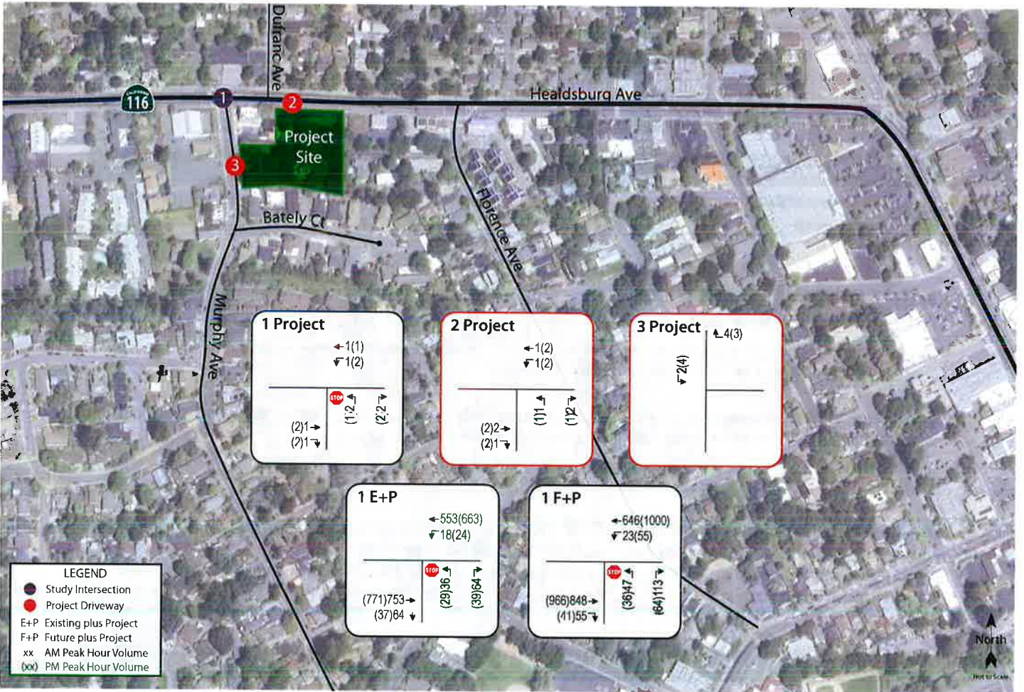
Traffic Study for the Pacific Knolls Project Figure 3 – Project, Existing plus Project, and Future plus Project Traffic Volumes
