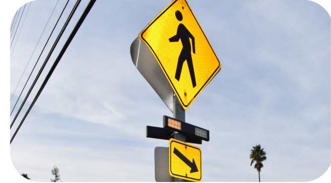
Rectangular Rapid Flashing Beacon
