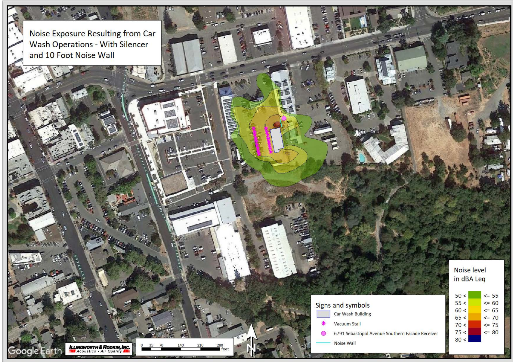
FIGURE 8 Noise Exposure Resulting from Car Wash Operations – With Silencer and 10ft Noise Wall
