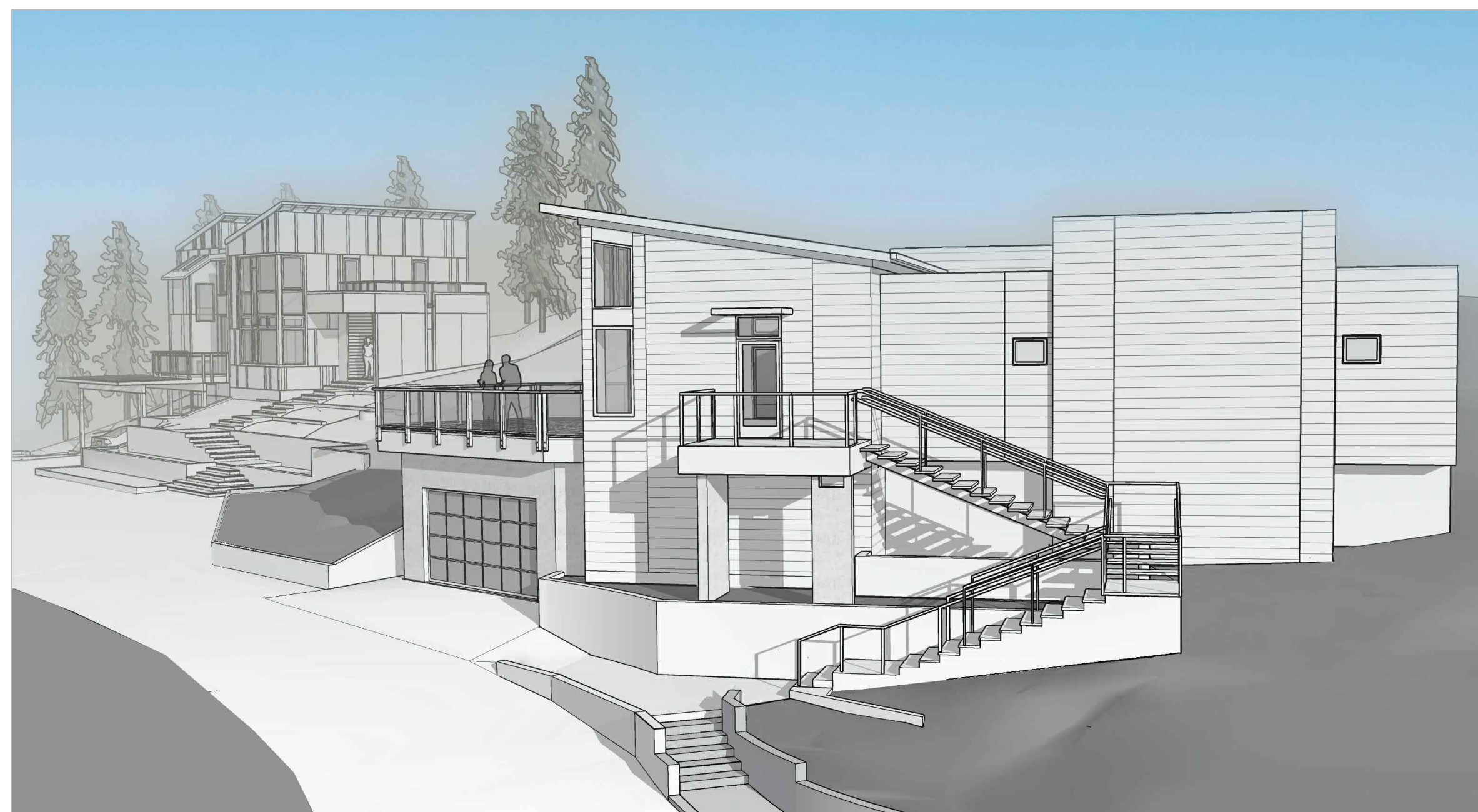
Garage, Stair and Entry Deck to break up massing Tallest vertical surface to highlight the Entry Secondary vertical to be a backdrop to landscape elements Lower rooflines add horizontal contrast to the pavilion forms
